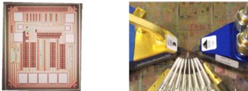
Figure 21: 140GHz VCO microphotograph and the measurements on wafer set up at IEMN, France
