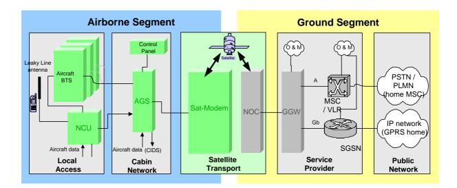
Architecture of the GSM onboard system
